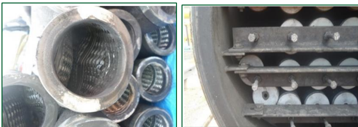
Figure 2. Example of (a) Collapsed elements (left) and (b) Bypassed elements
