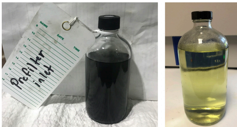
Figure 6. Sour water feed prior to the TORSEP system (left) and after (right).
