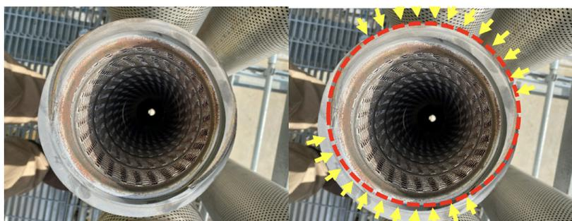
**Figure 4.** Sealing surface of the dust filters. The picture on the left shows the groove of the 'knife edge' sealing surface. The picture on the right illustrates the regions where the elastomer does not seal.
