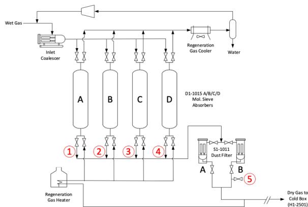
**Figure 2.** Process flow diagram indicating analysis locations.
