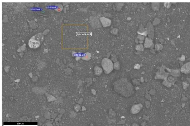
**Figure 3.** Scanning electron micrograph of contaminant entering the cryogenic exchanger.
