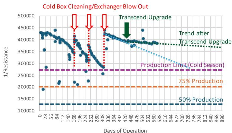
**Figure 5.** Heat transfer resistance over time, showing the impact of the Transcend upgrade.
